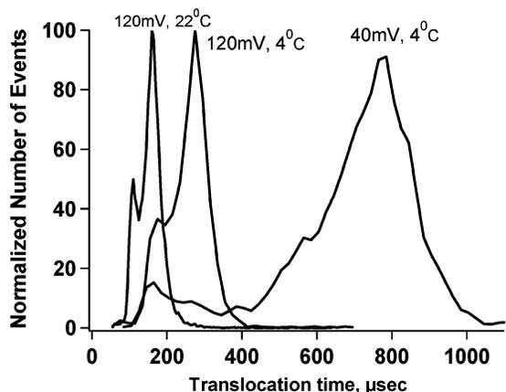
**Figure 4.** Translocation time is increased when the temperature is decreased. At low voltage (40 mV) and low temperature (4 °C) in 1.6 M KCl-TE containing 20% glycerol, the translocation time is about 800  $\mu$ s.
