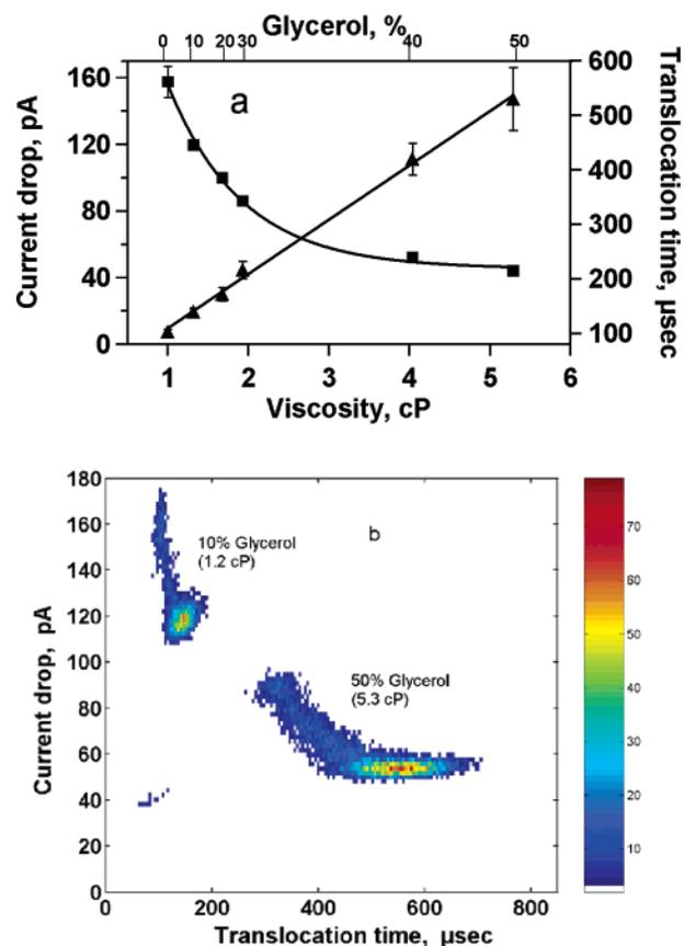
**Figure 1.** (a) Current blockage (■) and translocation time (▲) versus viscosity for 3 kbp DNA in 1.5 M KCl-TE solution at 120 mV bias voltage. The solid curves are fits for  $\Delta I_b \sim 1/\eta$  and  $t_d \sim \eta$ . (b) The scatter plots for the addition of 10% and 50% glycerol to the ionic solution. The color scale represents the events density.
