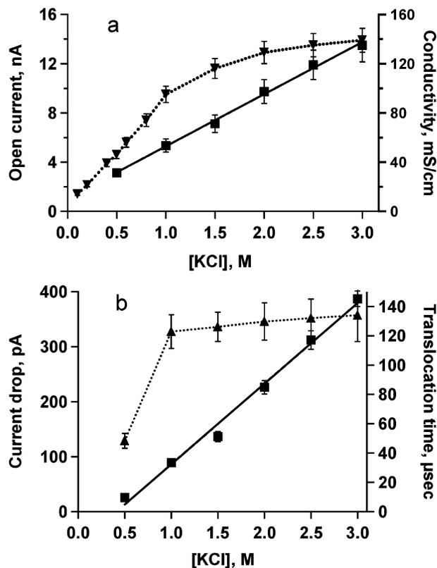
**Figure 3.** (a) Open current (■) (without DNA added) and bulk conductivity (▲) change as a function of salt concentration at 120 mV bias voltage. (b) Current drop (■) and translocation time (▲) change as a function of KCl concentration. The solid curves are linear fits of  $\Delta I_b$  and  $t_d$  to KCl concentration.
